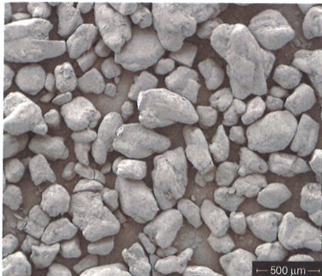
SEM 2: Excipient: boric acid; manufacturer: Aldrich Chemical Company Inc.; lot no.: 01559BU; magnification: 100×; voltage: 5 kV.
