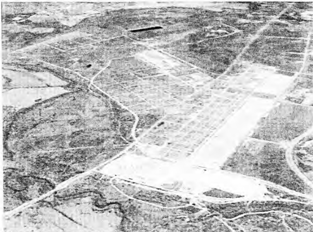
Figure 4. Geographically specific satellite imagery is applied to the terrain polygons in patches. Multiple patch sizes are encoded into the database for varying levels of detail. This image is a B/W screen capture from the real time image generator.
