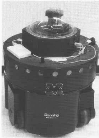
Figure 2-22. The Denning MRV-2 mobility base incorporates a three-point synchro-drive configuration with each wheel located directly below the pivot axis of the associated steering column (courtesy Georgia Institute of Technology).
