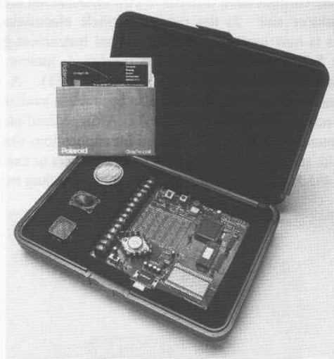
Figure 5-6. The Polaroid Ultrasonic Ranging Developer's Kit offers programmable pulse, frequency, and gain parameters, with the ability to detect multiple echoes (courtesy Polaroid Corp.).
