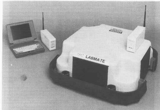
Figure 3-6. The tactile bumper employed on the LabMate uses a conductive foam material separated from a flexible metal backplate by an insulating mesh (courtesy Transitions Research Corp.).
