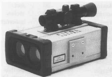
Figure 5-18. The Class 1 (eye-safe) LD90-3 series TOF laser rangefinder is a self-contained unit available in several versions with maximum ranges of 150 to 500 meters under average atmospheric conditions (courtesy RIEGL USA).
