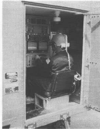
Figure 1-15. The TOV Control Van consists of a HMMWV-mounted environmental shelter containing three operator control stations and a fourth supervisor station (courtesy Naval Command Control and Ocean Surveillance Center).
