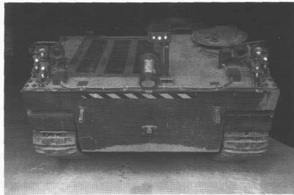
Figure 2-10. A commercially available John Deere agricultural ground-speed sensor was employed on the Ground Surveillance Robot to improve dead-reckoning accuracy (courtesy Naval Command Control and Ocean Surveillance Center).
