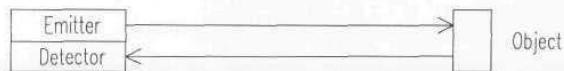
Figure 3-28. Diffuse-mode proximity sensors rely on energy reflected directly from the target surface.
