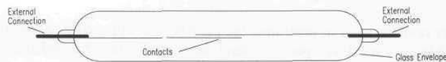
Figure 3-8. The hermetically sealed magnetic reed switch , shown here with normally open contacts, is filled with inert gas and impervious to dust and corrosion.
