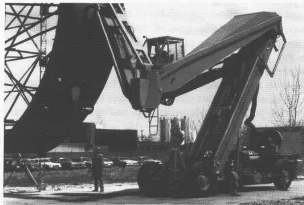
Figure 3-22. This robotic shot-blasting device employs inductive proximity sensors to keep the closed-cycle end-effector in sealed contact with the ship's hull (courtesy Barnes and Reineke).
