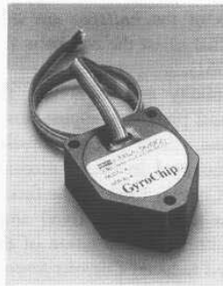
Figure 13-2. The GyroChip solid-state gyro employs a double-ended quartz tuning fork (courtesy Systron Donner Inertial Division).
