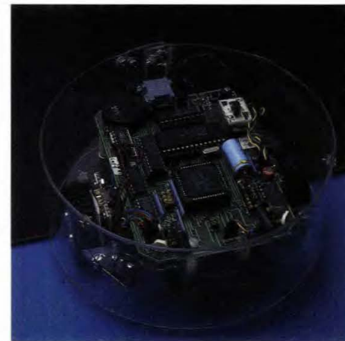
The Rug Warrior class of robots are microprocessor-controlled and have ten sensors and two motor drivers onboard. Rug Warrior I here has a cylindrical bump skirt for detecting collisions and is driven by two motors in a differential manner.
