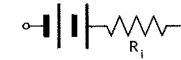
Figure 8.4: A battery may be modeled as an ideal battery, one able to supply any current at constant voltage, in series with an internal resistance, R_i .
