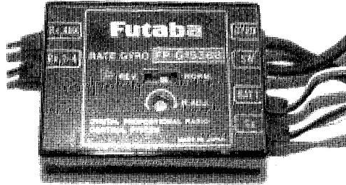
Figure 5.32: Futaba makes a small, rate gyro for model airplanes. The input is a pulse-width-modulated signal, and the output is an increased or decreased pulse width, depending on the rate of rotation.
