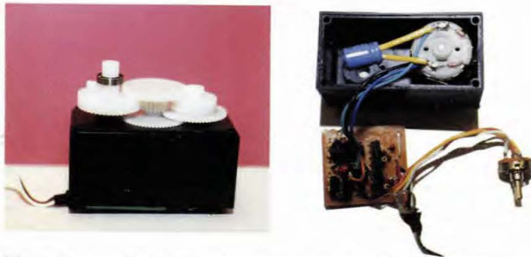
These photographs illustrate the internals of a Royal Titan Maxi servo motor. At left, the top cover of the servo motor is removed, revealing the gear train. At right is a bottom view of the motor casing which shows the DC motor, the potentiometer, and the control circuit.
