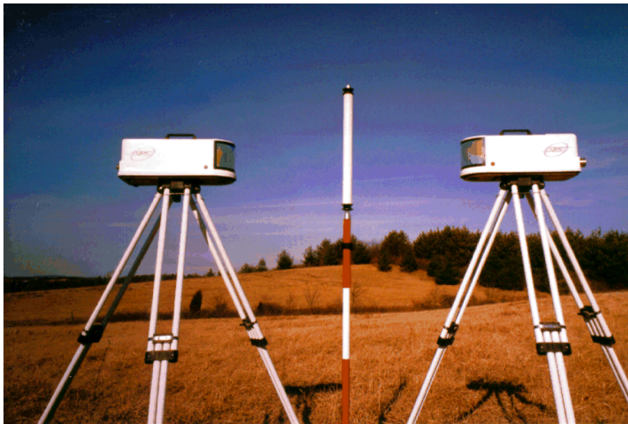
Figure 6.26: The Odyssey positioning system comprises two laser beam transmitters and a pole- or wand-mounted receiver. (Courtesy of Spatial Positioning Systems, Inc.)
