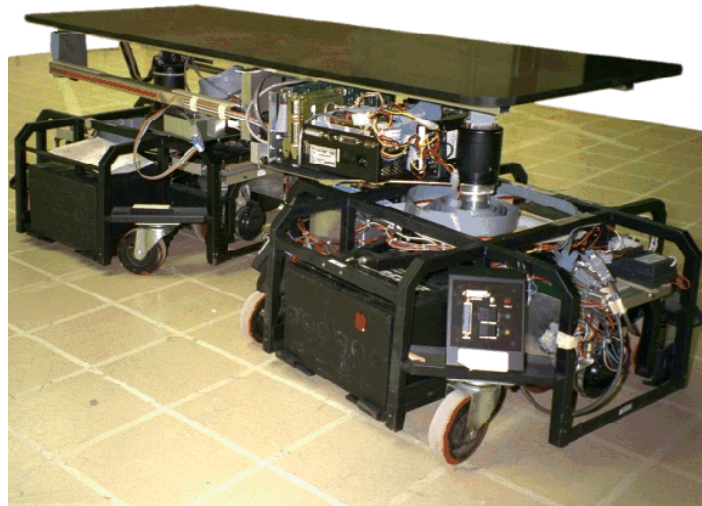
Figure 1.16: The University of Michigan's MDOF vehicle is a dual-differential-drive multi-degree-of-freedom platform comprising two TRC LabMates . These two "trucks" are coupled together with a compliant linkage , designed to accommodate momentary controller errors that would cause excessive wheel slippage in other MDOF vehicles. (Courtesy of The University of Michigan.)
