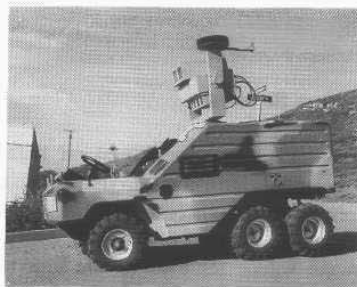
Figure 17-6. The Surrogate Teleoperated Vehicle (STV) developed by Robotic Systems Technologies employs a 360-degree acoustical sensing array (top-left of mast) manufactured by SAIC Bio-Dynamics (courtesy Naval Command Control and Ocean Surveillance Center).
