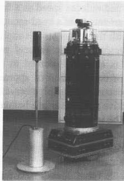
Figure 15-10. ROBART II approaches its automatic recharging station by homing in on the active near-infrared beacon shown at the top of the support pole.
