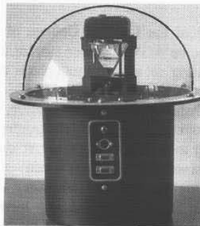
Figure 15-18. The EZNav Position Sensor can process up to 32 separate beacon targets per scan, with a complete X-Y position update computed at a 10-Hz rate (courtesy Intelligent Solutions, Inc.).
