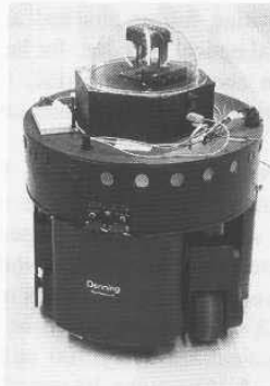
Figure 15-19. The earlier Lasernav prototype is used by Georgia Tech as the primary navigational referencing sensor on a Denning MRV-2 robotic base (courtesy Georgia Institute of Technology).
