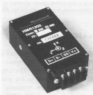
Figure 12-25. The Honeywell HMR-Series Smart Digital Magnetometer is a three-axis magneto-resistive magnetometer with a sensitivity of 1 milliGauss over a measurement range of \pm 1 Gauss (courtesy Honeywell Solid State Electronics Center).
