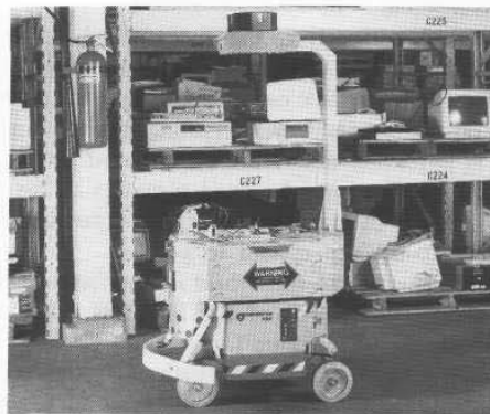
Figure 11-16. The MDARS Interior robot normally traverses virtual paths generated by the Cybermotion Dispatcher , switching to free-ranging off-path operation in the event of a perceived obstruction.
