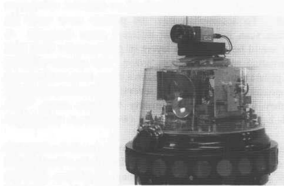
Figure 7-11. The near-infrared proximity sensor developed for ROBART II used a programmable array of four high-powered LED emitters with a variable threshold receiver. The PIN-photodiode detector is situated at the focal point of the parabolic reflector.
