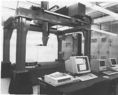
Figure 7-2. The CMS-1000 uses multiple HeNe laser beams to track retroreflective targets attached to the moving end effector of the Intelligent Robotic Inspection System built for the Navy by MTS Systems Corp. (courtesy Applied Research Lab, Penn State University).
