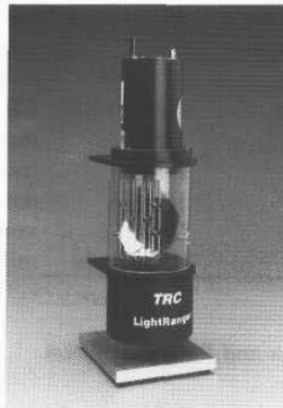
Figure 6-20. The TRC Light Direction and Ranging System incorporates a two-axis scanner to provide full-volume coverage sweeping 360 degrees in azimuth and 45 degrees in elevation (courtesy Transitions Research Corp.).
