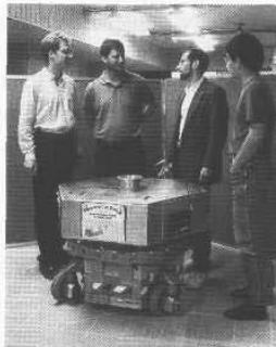
Figure 10-13. CARMEL, developed by the University of Michigan, incorporates a Cybermotion K2A Navmaster base outfitted with a ring of 24 Polaroid ultrasonic rangefinders (courtesy University of Michigan).
