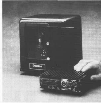
Figure 6-11. The Odetics Scanning Laser Imaging System captures a 128- by 128-pixel image every 835 milliseconds (courtesy Odetics, Inc.).
