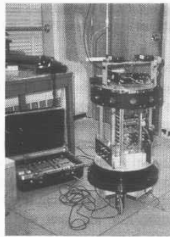
Figure 10-3. Brooks (1986) applied the classical potential field method to an autonomous mobile robot equipped with a ring of 12 Polaroid ranging sensors (courtesy MIT AI Lab).
