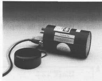
Figure 6-18. The AccuRange 3000 distance measuring sensor provides a square-wave output that varies inversely in frequency as a function of range (courtesy Acuity Research, Inc.).
