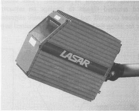
Figure 6-8. The LASAR 3-D scanner achieves a range-measurement accuracy of 2 millimeters over a 45- by 45-degree field of view at a stand-off distance of 2 meters (courtesy Perceptron Corp.).
