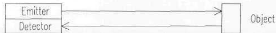
Figure 3-28. Diffuse-mode proximity sensors rely on energy reflected directly from the target surface.
