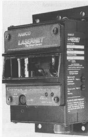
Figure 4-28. The Lasernet ® system detects retroreflective targets with a scanning near-infrared laser to provide bearing and range information used in the navigation of automated guided vehicles (courtesy NAMCO Controls).
