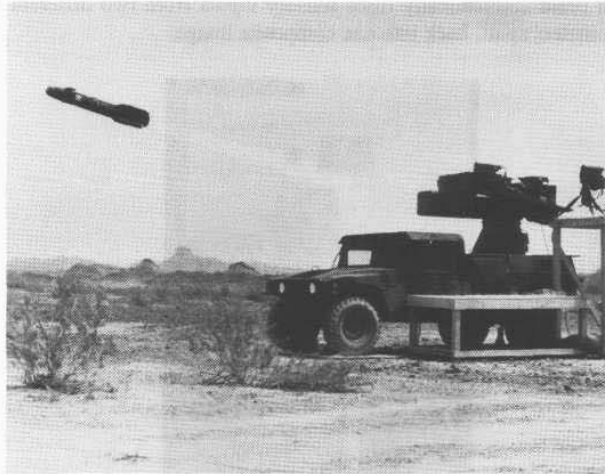
Figure 1-17. A Rockwell Hellfire missile comes off the rail in response to a remote command from the TOV operator located in the Control Van several kilometers away during demonstrations for a high-level Department of Defense audience at Camp Pendleton, CA, in September 1989 (courtesy Naval Command Control and Ocean Surveillance Center).
