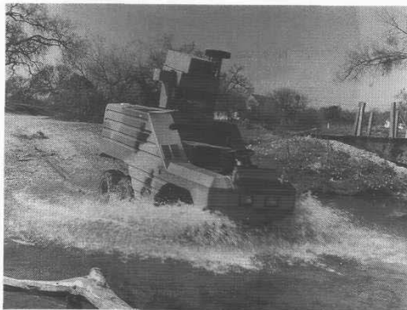
Figure 1-21. Shown here crossing a stream at Fort Hunter Liggett, the Surrogate Teleoperated Vehicle is capable of traversing through water up to 2 feet deep (courtesy Unmanned Ground Vehicle Joint Program Office).
