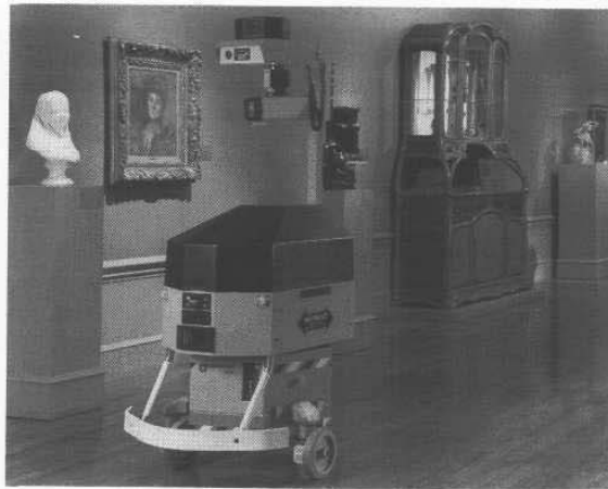
Figure 3-7. The tactile bumper on the Cybermotion K2A Navmaster robot is configured to activate adjustable-threshold strain sensors in the left and right supporting arms (courtesy Cybermotion, Inc.)
