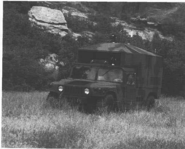
Figure 4-9. The JPL stereo vision system was used to detect obstacles for the HMMWV-based Surrogate Semiautonomous Vehicle (SSV) at Demo B in June 1994 (courtesy Martin Marietta Denver Aerospace).
