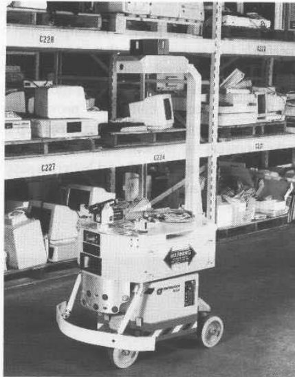
Figure 1-20. The MDARS Interior robot equipped with the Cybermotion SPI Module on patrol in the Camp Elliott warehouse in San Diego, CA (courtesy Naval Command Control and Ocean Surveillance Center).
