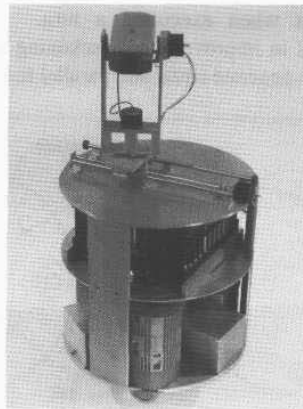
Figure 2-21. The CMU robot Pluto employs three electronically synchronized drive wheels (courtesy Carnegie Mellon University).
