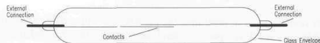
Figure 3-8. The hermetically sealed magnetic reed switch , shown here with normally open contacts, is filled with inert gas and impervious to dust and corrosion.
