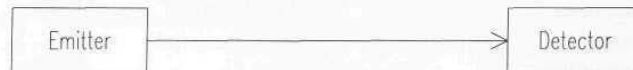
Figure 3-25. The opposed-mode sensor configuration relies on target passage between the emitter and detector to interrupt the beam.
