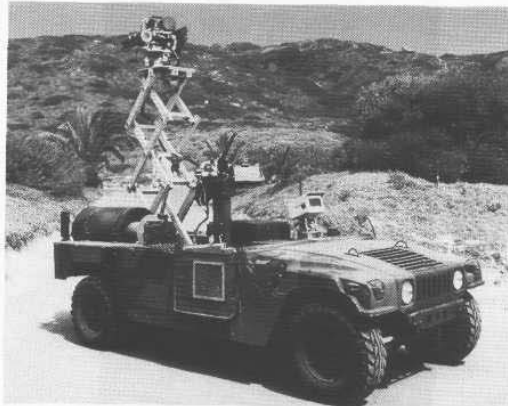
Figure 1-14. One of three remotely driven reconnaissance, surveillance, and target acquisition (RSTA) vehicles developed by NCCOSC for the USMC TeleOperated Vehicle (TOV) program (courtesy Naval Command Control and Ocean Surveillance Center).
