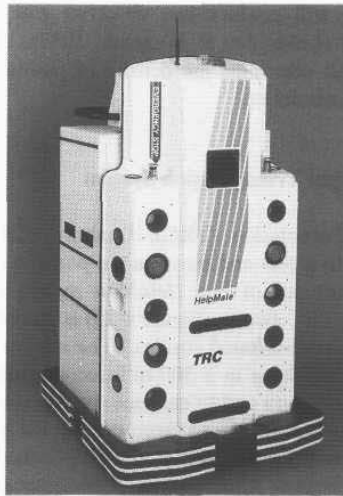
Figure 4-26. Slots for the two structured-light strobes are visible directly above and below the company's logo on the front panel of TRC HelpMate (courtesy Transitions Research Corp.).
