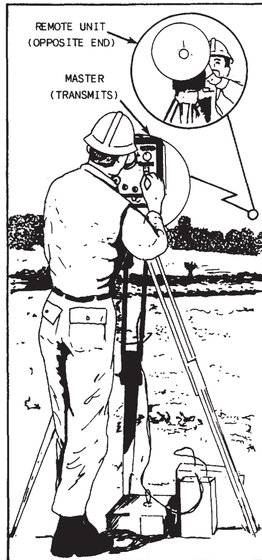
Figure 12-24.-Setting a microwave distance-measuring unit.
