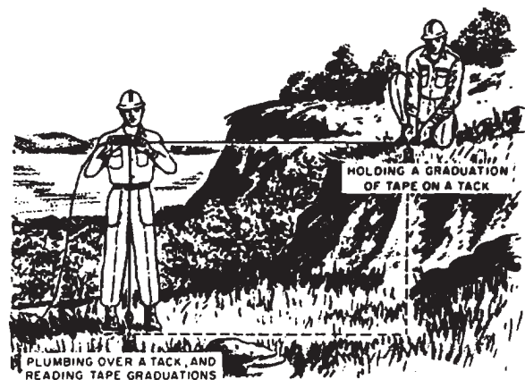
Figure 12-12.-Horizontal taping on a slope.
