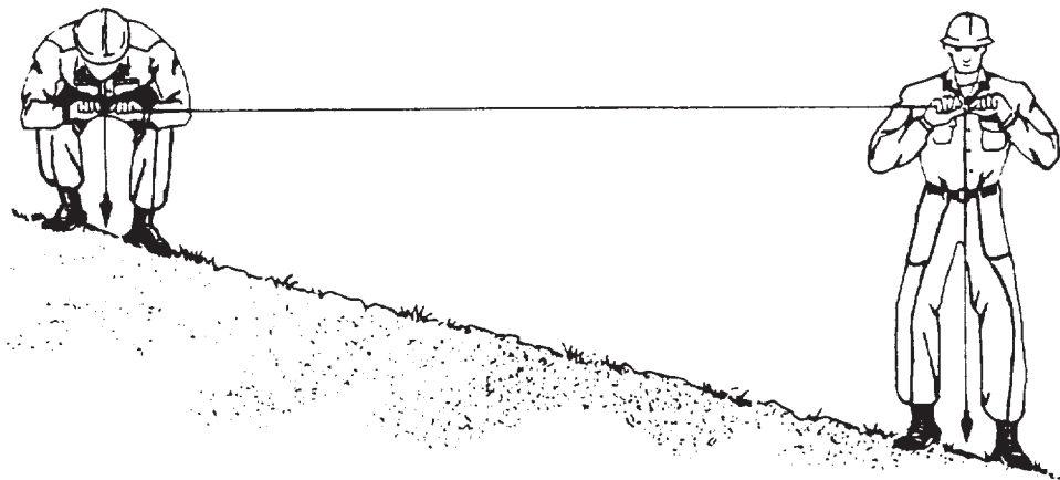
Figure 12-13.—Horizontal chaining using plumb bobs.
