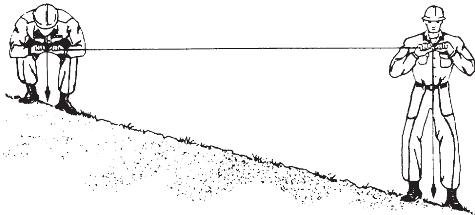
Figure 12-13.—Horizontal chaining using plumb bobs.
