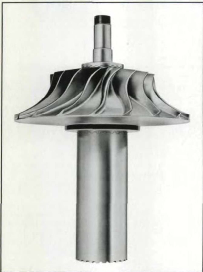
Fig. 4—A stationary gas turbine rotor showing the through bolts used for clamping the Fixed Curvic Coupling members together.
