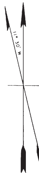
Figure 11-1.-An orientation symbol or meridian arrows.
