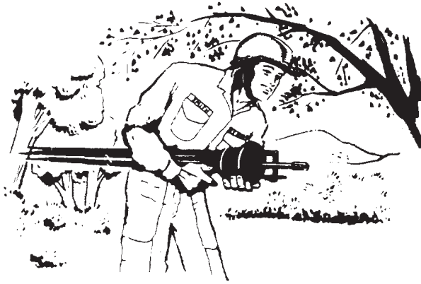
Figure 14-4. Recommended carrying position of instrument when obstacles may be encountered.
