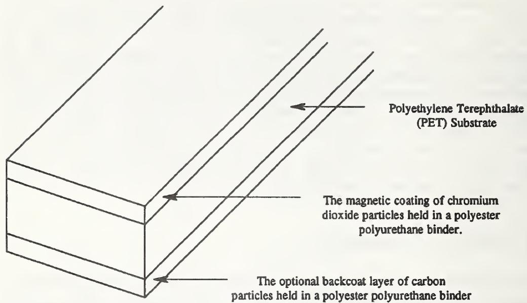
**Figure 1. 3480 Type Tape Structure.**
