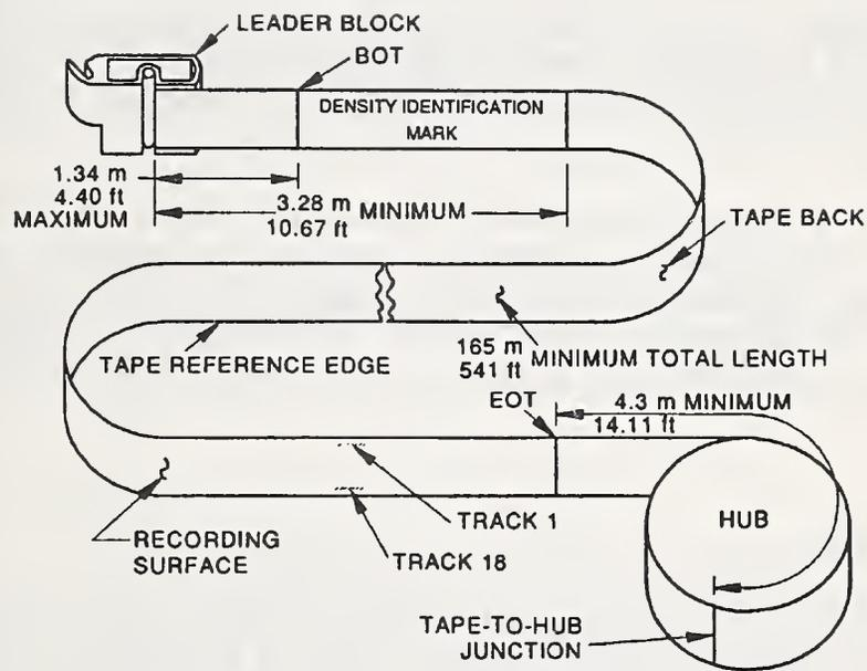
**Figure 4. 3480 Type Tape Usable Recording Area.**
