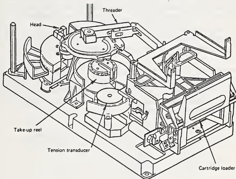
**Figure 3. 3480 Type Tape Drive Assembly.**
