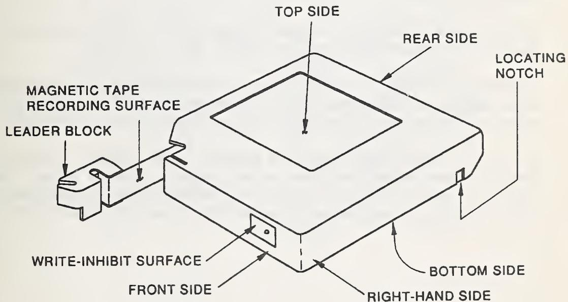
**Figure 2. 3480 Type Tape Cartridge Assembly.**
