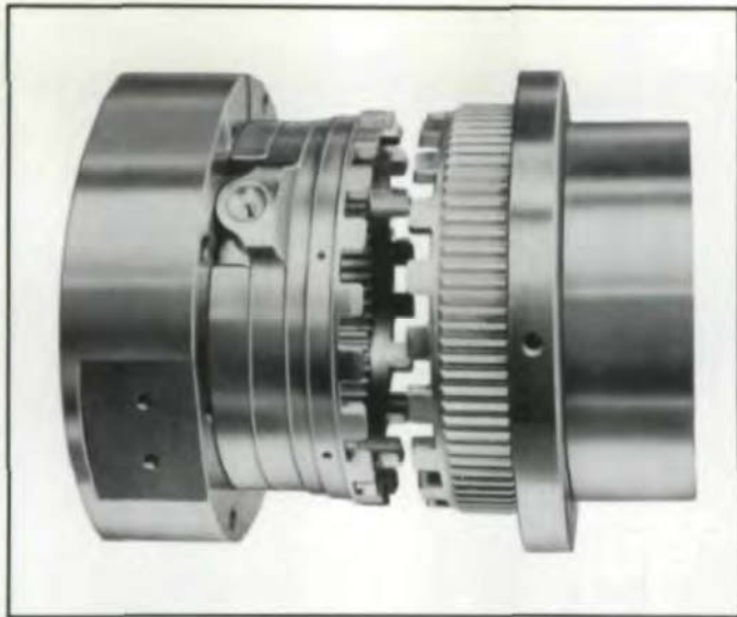
Fig. 10 - A Curvic Coupling of the semi-universal type is employed at both ends of this intermediate drive shaft.
