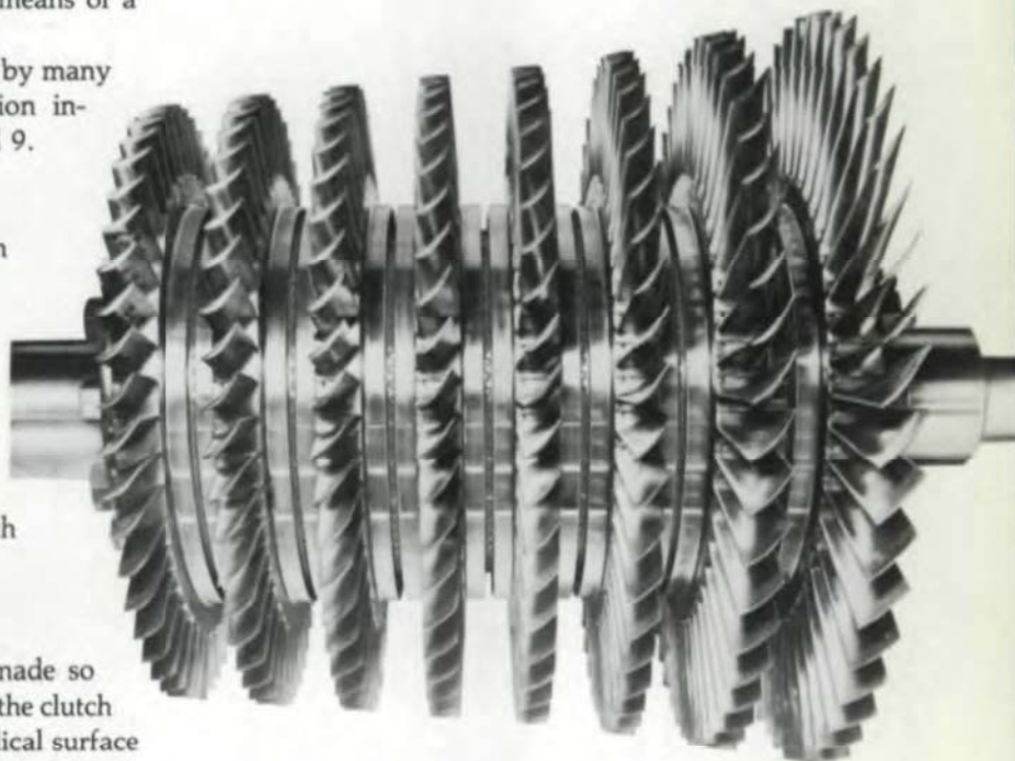
Fig. 3—A turbine rotor assembly for a stationary gas turbine. Note the Fixed Curvic Coupling teeth between each disc.
