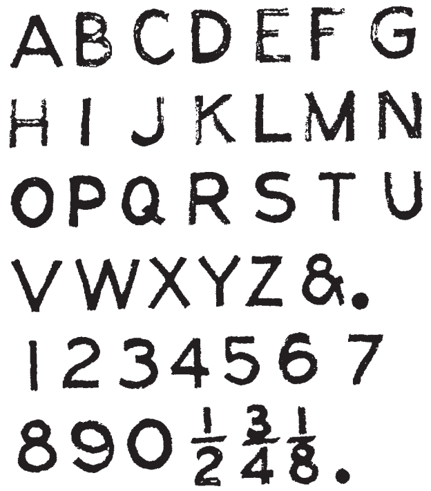
Figure 3-45.-Vertical single-stroke Gothic capitals and numerals.
