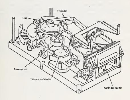
Figure 3. 3480 Type Tape Drive Assembly.
