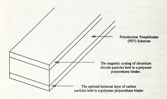
Figure 1. 3480 Type Tape Structure.
