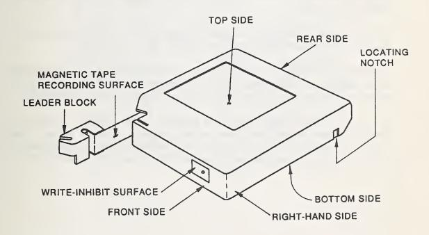
Figure 2. 3480 Type Tape Cartridge Assembly.
