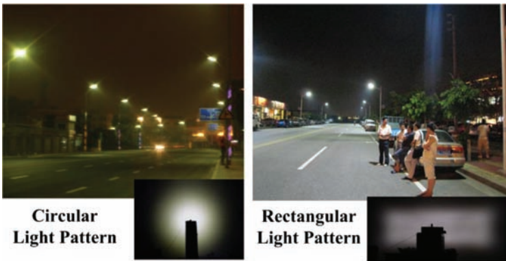
Figure 6.3 A comparison of road lighting performances of two LED road lights with circular light pattern and rectangular pattern respectively. (Color version of this figure is available online.)
