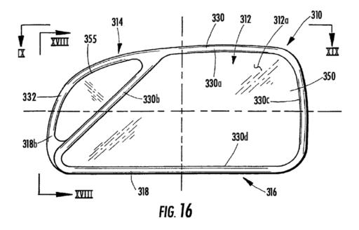
Figure 16 of the '882 patent, reproduced above, shows an embodiment of a plano reflective element assembly. Ex. 1001, 4:22–23.
