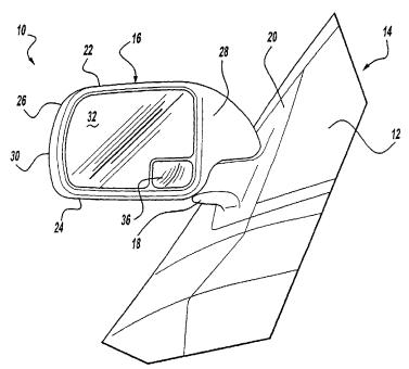
(57) Abstract: A mirror assembly (10) in which a mirror housing (16) and multi-function backing plate (34) provides various useful functions. The multi-function backing plate supports not only a conventional reflective element (32) but also supports a wide angle reflective element (36). The multi-function backing plate further supports an indicator light assembly (96) so that the mirror assembly can provide an indicator light function.
