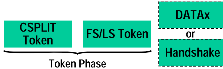
Figure 8-7. Packets in a Complete-split Transaction
