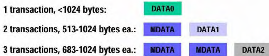
Figure 5-12. Data Phase PID Sequence for Isochronous OUT High Bandwidth Endpoints
