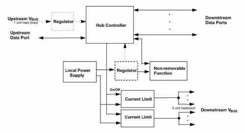
Figure 7-43. Compound Self-powered Hub
