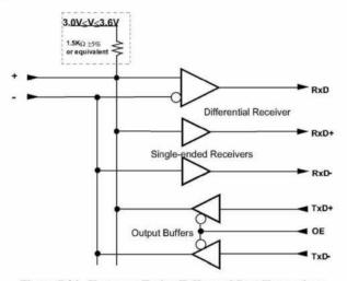
Figure 7-24. Upstream Facing Full-speed Port Transceiver
