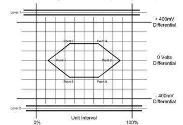
Figure 7-14 shows transmit waveform requirements for a device (with a captive cable) measured at TP2.
