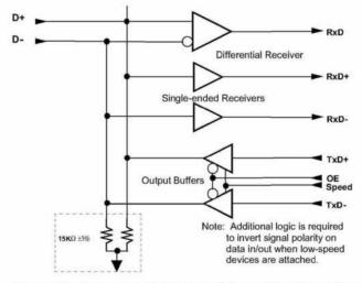
Figure 7-25. Downstream Facing Low-/full-speed Port Transceiver
