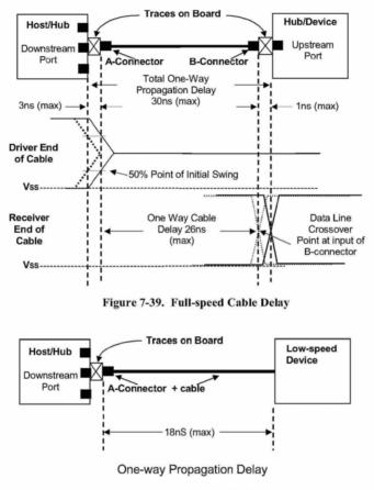
Figure 7-40. Low-speed Cable Delay
