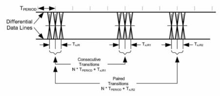
Figure 7-51. Receiver Jitter Tolerance for Low-/full-speed
