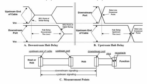
Figure 7-38. Hub Propagation Delay of Full-speed Differential Signals
