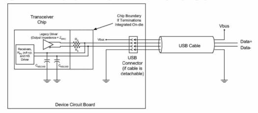
Figure 7-23. Diagram for High-speed Loading Equivalent Circuit
