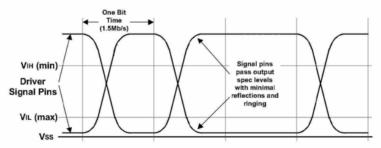
Figure 7-7. Low-speed Driver Signal Waveforms
