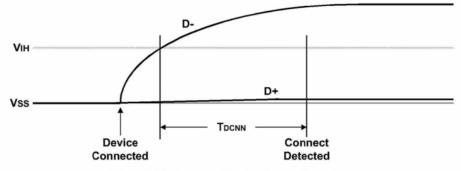
Figure 7-28. Low-speed Device Connect Detection
