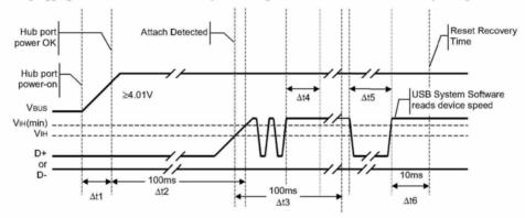
Figure 7-29. Power-on and Connection Events Timing
