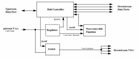
Figure 7-42. Compound Bus-powered Hub
