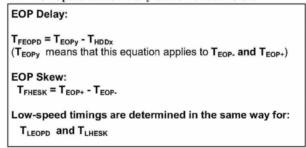
Figure 7-53. Hub EOP Delay and EOP Skew for Low-/full-speed
