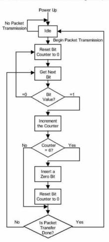
Figure 7-34. Flow Diagram for Bit Stuffing
