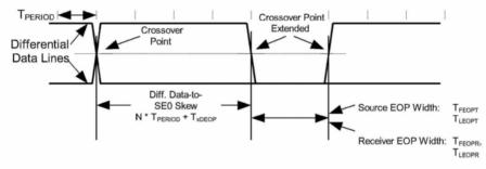
Figure 7-50. Differential-to-EOP Transition Skew and EOP Width for Low-/full-speed
