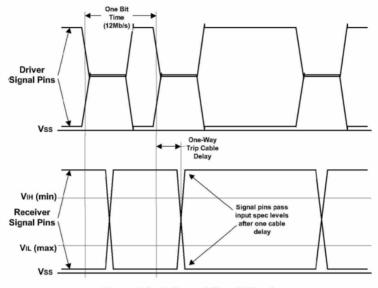
Figure 7-6. Full-speed Signal Waveforms
