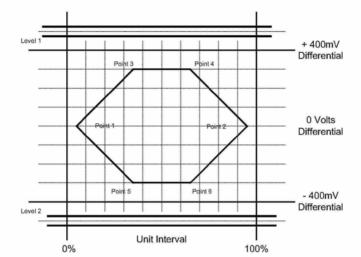
Figure 7-17 shows transmit waveform requirements for a hub transceiver measured at TP1 and for a device transceiver measured at TP4.
