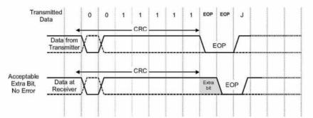
Figure 7-33. Illustration of Extra Bit Preceding EOP (Full-/low-speed)
