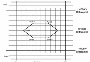
0% Unit Interval 100% Voltage Level (D+ - D-) Time (% of Unit Interval) Level 1 575 mV N/A Level 2 -575 mV N/A Point 1 0 V 15% UI Point 2 0 V 85% UI Point 3 150 mV 35% UI Point 4 150 mV 65% UI Point 5 -150 mV 35% UI Point 6 -150 mV 65% UI
