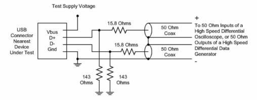
Figure 7-12. Transmitter/Receiver Test Fixture
