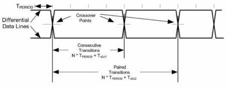
Figure 7-49. Differential Data Jitter for Low-/full-speed
