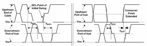
A. Downstream EOP Delay with Cable
