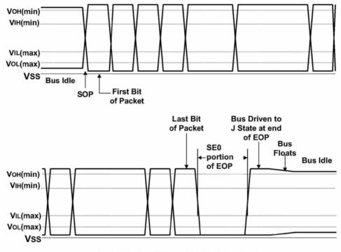
Figure 7-30. Low-/full-speed Packet Voltage Levels
