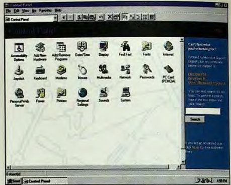
Internet Explorer 4.0's Web view of the Control Panel. The frame on the right shows an associated HTML help text.
