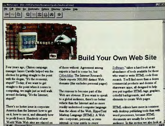
Netscape Navigator supports tags that will automatically flow text into multiple columns.
