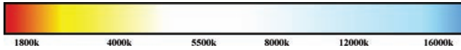
Figure 3.10 Colors corresponding to different color temperatures. (Color version of this figure is available online.)
