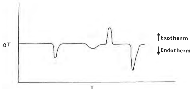
FIGURE 18. A DTA thermogram showing the changes that occur upon heating the compound H1.
