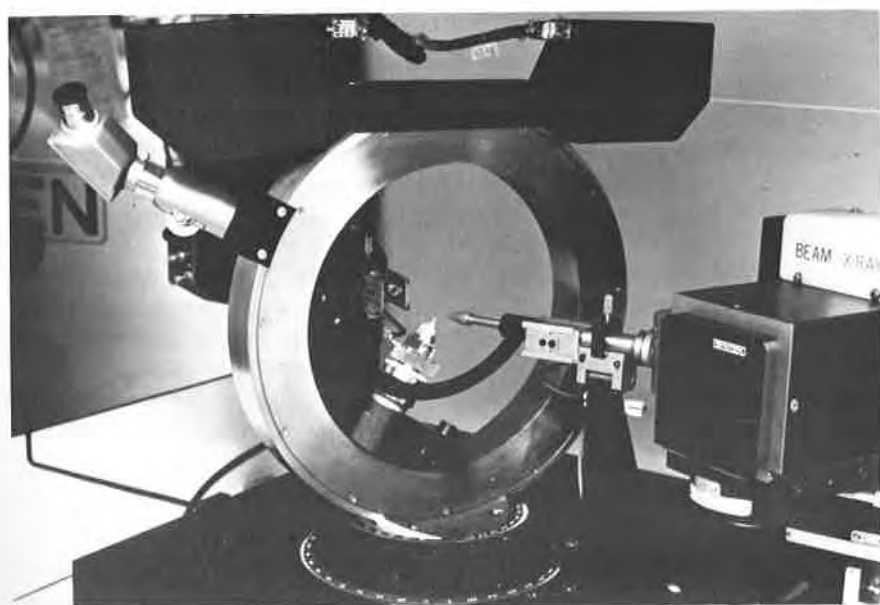
FIGURE 8. The chi circle of an automated x-ray diffractometer.
