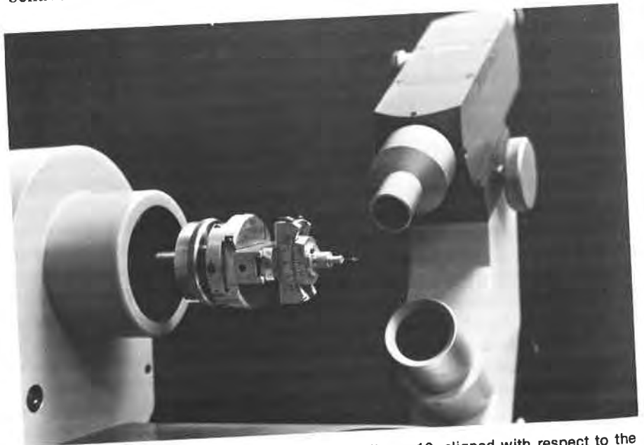
FIGURE 11. The same crystal as shown in Figure 10, aligned with respect to the spindle axis.
