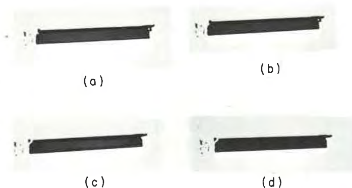
FIGURE 13. Desolvation of a crystal of bis(salicylaldehyde)ethylenediimine cobalt(II) chloroformate with its ends removed at room temperature: (a) at start; (b) after 12 hr; (c) after 28 hr; and (d) after 48 hr. The long axis of the crystal is the b crystallographic axis.
