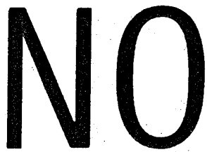
Figure 2a. Etched chrome on glass: Stairstepping = 30
