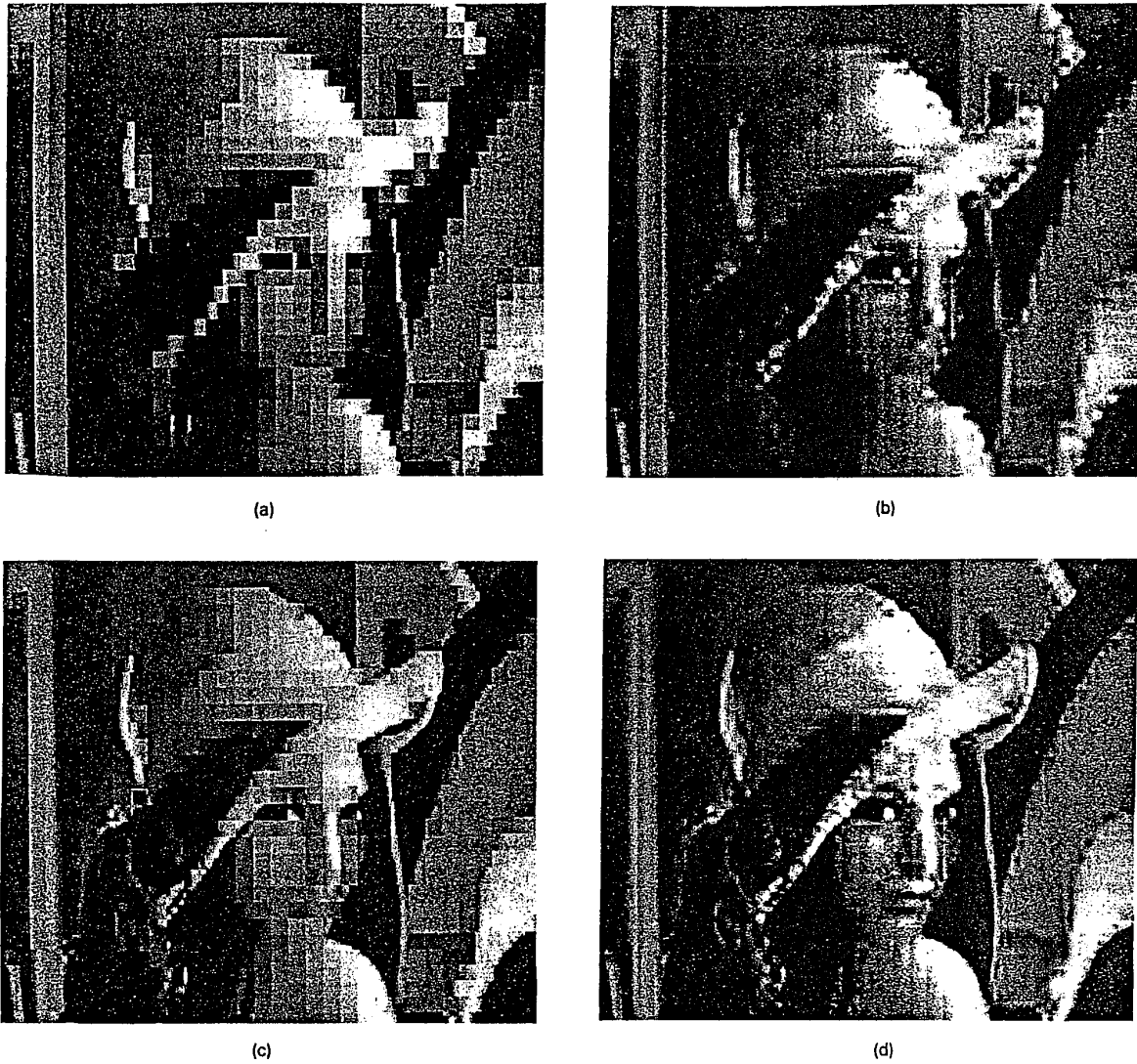
Fig. 13 Partially reconstructed images: (a) DCT 0.2 bit/pel, (b) LOT 0.2 bit/pel, (c) DCT 0.3 bit/pel, and (d) LOT 0.3 bit/pel.
