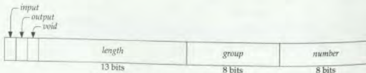
Figure 17.19 The structure of an ioctl command.
