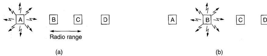
Fig. 4-11. A wireless LAN. (a) A transmitting. (b) B transmitting.
