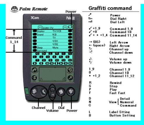
The Graffiti command, the application launcher buttons, and the scroll buttons under the graffiti area can also be used.
