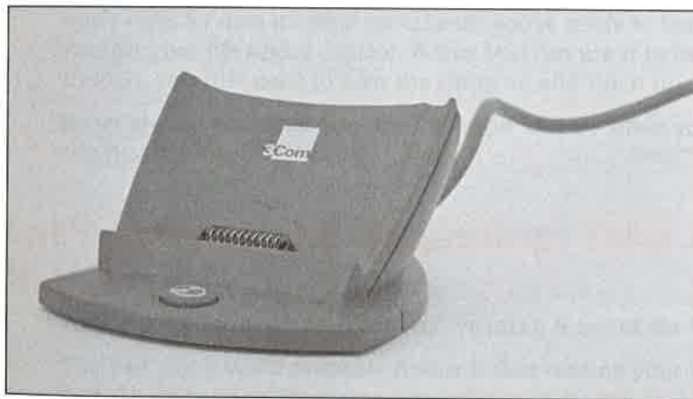
The cradle lets you synchronize the information between your PalmPilot and your computer.
