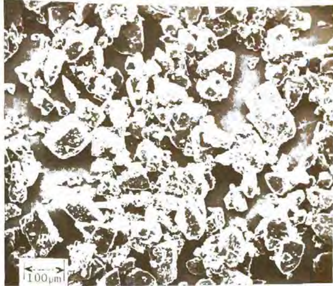
SEM: 7 Excipient: Lactose monohydrate ( Lactose Monohydrate Capsulating ) Manufacturer: Quest International Inc. (Sheffield Products) Lot No.: 58A-10 (9 NL 20) Magnification: 120 × Voltage: 20 kV
