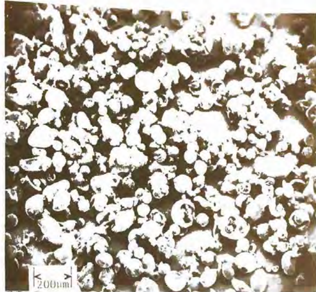
SEM: 7 Excipient: Povidone K-29/32 (Plasdone K-29/32) Manufacturer: ISP Lot No.: 82A-3 Magnification: 60 × Voltage: 5 kV
