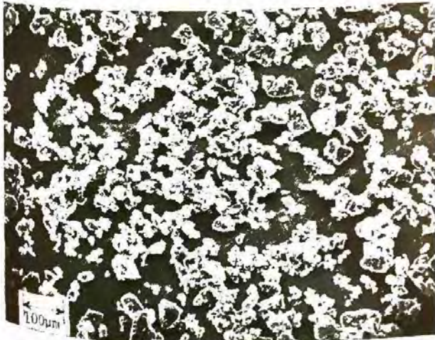
SEM: 6 Excipient: Lactose monohydrate ( Lactose Monohydrate 80M ) Manufacturer: Quest International Inc. (Sheffield Products) Lot No.: 58A-11 (9 NL 18) Magnification: 120 × Voltage: 20 kV
