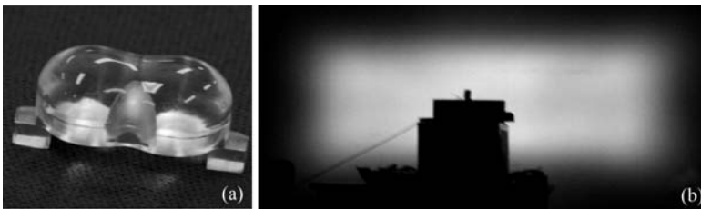
Figure 6.61 (a) Continuous freeform lens for LED road lighting; and (b) its illumination performance in laboratory.
