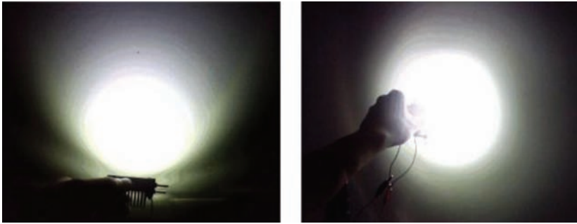
Figure 3.58 Illustration of yellow ring in LED modules. (Color version of this figure is available online.)
