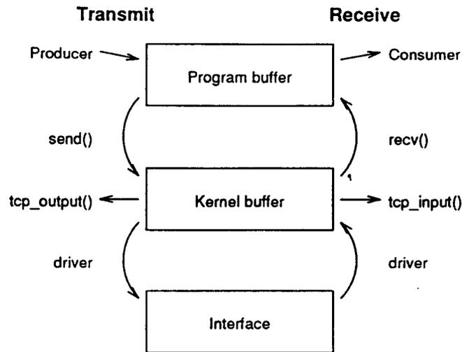
Figure 1: *Data movements in a typical TCP/IP implementation*
