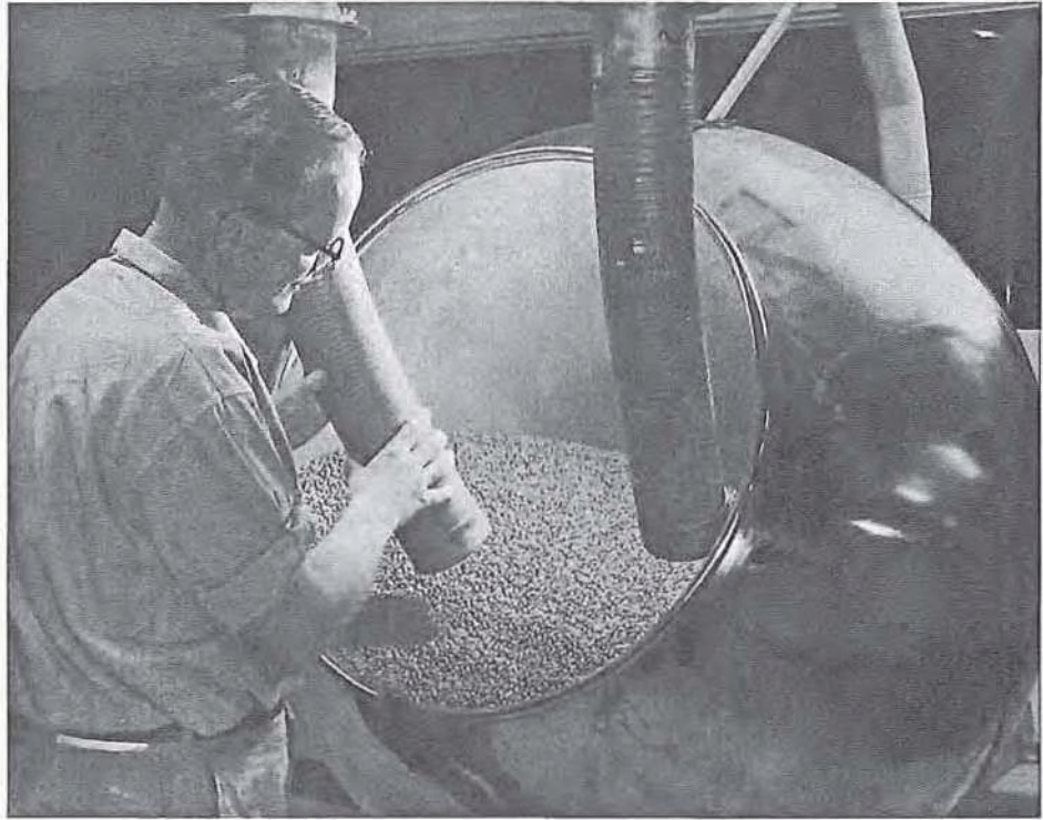
Fig. 5-50. Tablet coating, an older style coating pan, showing the warm air supply and the exhaust. (Courtesy of Wyeth Laboratories.)
