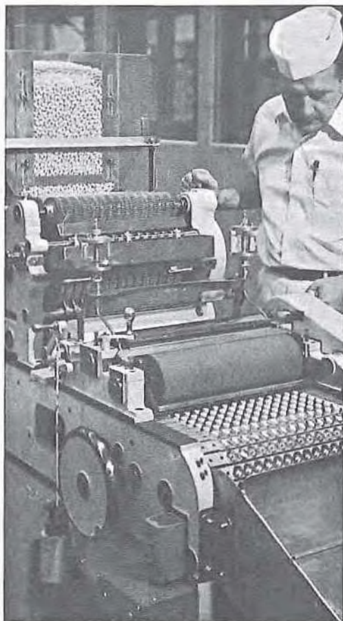
Fig. 5-53. Branding of coated compression tablets on a Hartnett branding machine. (Courtesy of The Upjohn Company.)
