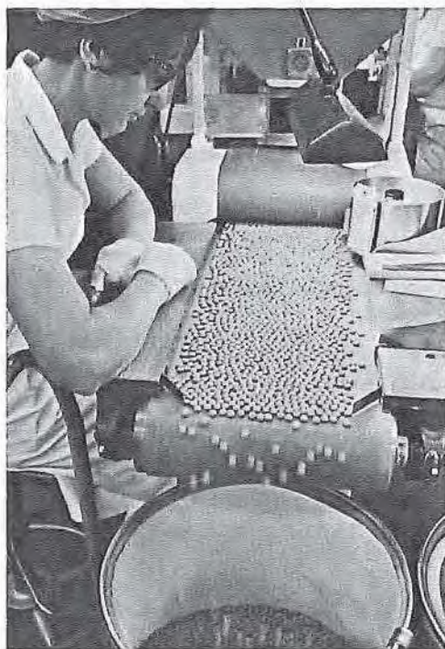
Fig. 5-57. Checking for physical imperfections in coated tablets. (Courtesy of Smith, Kline & French.)
