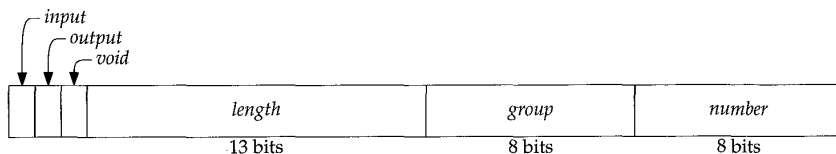
Figure 17.19 The structure of an ioctl command.
