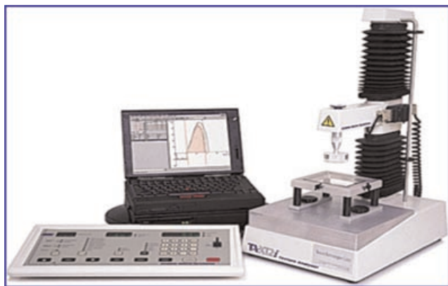
Figure 1. TA.XT2i Texture Analyzer (from Texture Analyzer Corp., Scarsdale, NY) used for bioadhesivity testing of the nail lacquer formulations.
