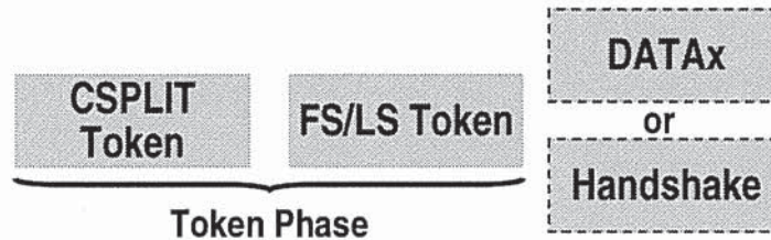
Figure 8-7. Packets in a Complete-split Transaction
