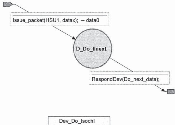
Figure 8-43. Isochronous IN Transaction Device State Machine
