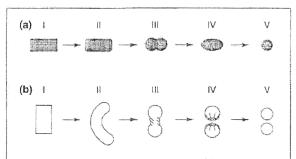
Figure 2. Pellet-forming mechanism according to: (a) Rowe<sup>36</sup> – I. Cylinder: II. Cylinder with rounded edges; III. Dumb-bell; IV. Ellipse; V. Sphere. (b) Baert – I. Cylinder; II. Rope; III. Dumb-bell; IV. Sphere with a cavity outside; V. Sphere. [Reproduced with permission from Ref. 9.]
