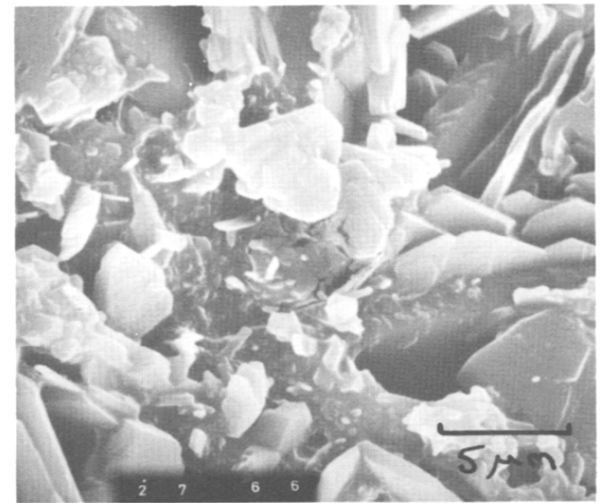
Fig. 3. Scanning electron micrographs of a Celutab particle (710 - 1000- \mu\text{m} sieve fraction).
