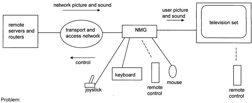
If television has been turned off using its remote control, how can we ensure that the network does not waste resources by continuing to send picture and sound to the NMG? That problem is solved with this invention.
