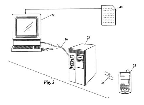
Figure 2 of the '748 patent is a diagram of system 10 as it is used for form creation. Ex. 1001, 6:58–59; 8:11–17. Computer 22 has an interface that allows a user to create and distribute a form to handheld devices using computer 22. *Id.* at 8:38–50. As the client enters questions and selects
