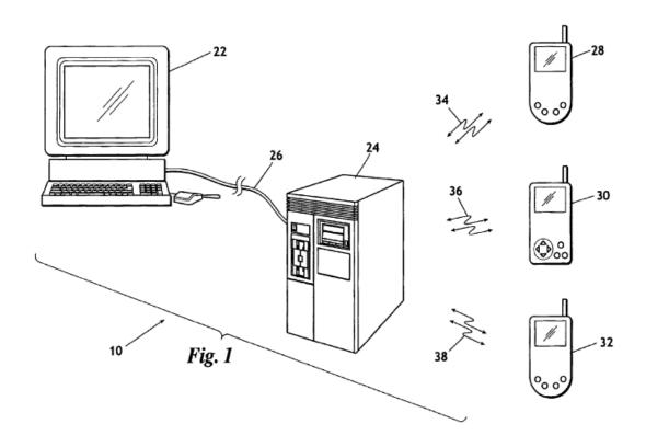
Figure 1 is a diagram of the '748 patent's system for data management. Ex. 1001, 6:57, 7:13–23. System 10 includes server 24; handheld computers 28, 30, and 32, which are operated remotely from server 24; and computer 22, which provides for administration of the system and reviewing data
