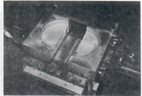
FIGURE 9. COMMERCIAL MOLD — SPLIT QUARTER MOLD SECTIONS
