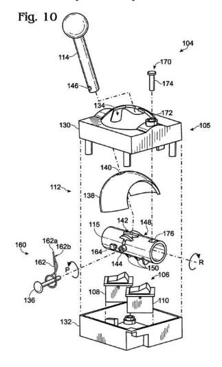
Figure 10 from the '850 patent is an exploded isometric view of a velocity control assembly, including actuator assembly 112.
