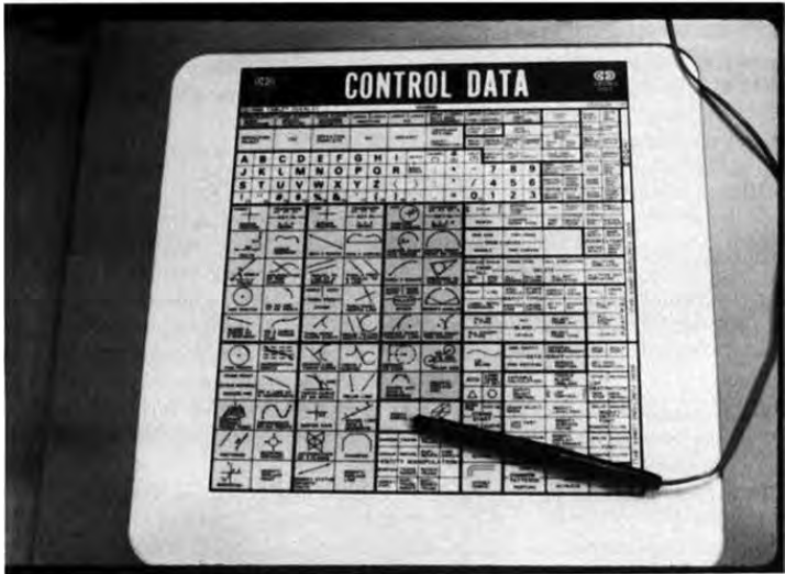
Figure 11. A data tablet overlay with command and keyboard entry areas. Notice the double coding of many commands with both a name and an icon.
