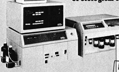
The 420A System is the first multifunctional, fully automated microanalyzer to eliminate sample contamination, degradation and loss associated with manual techniques. Thus, it delivers the highest sample-to-sample reproducibility, sensitivity and accuracy for the analysis of PTC amino acids and other derivatized biological compounds.
